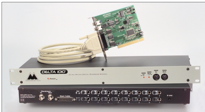
The rack-mount breakout box for M Audio's Delta 1010 contains all the converters and the TRS analog I/O jacks, as well as the word-clock and MIDI ports and the MIDI activity indicators. The audio ports are in the rear; the MIDI ports are, oddly, in the front. S/PDIF I/O is provided on the PCI card (top), which connects to the box via a standard DB-25 cable.
